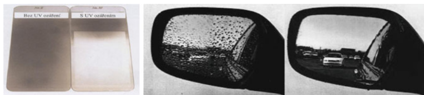
Fig. 2.18 Effects obtained by using photoactive TiO 2 (Hashimoto et al., 2005)
