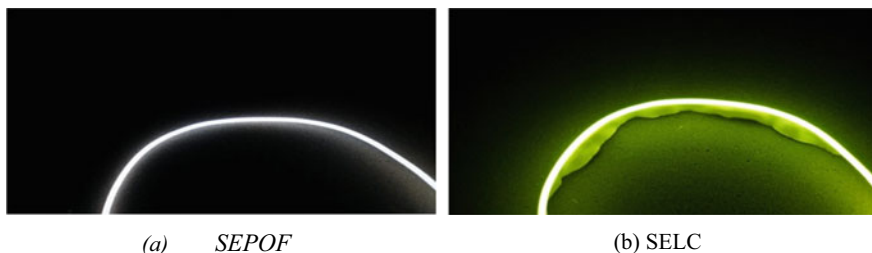
Fig. 5.18 Side emission of SEPOF and SELC (Mishra et al., 2013)
