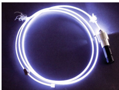
Fig. 5.14 Side-emitting POF with textile cover (Mishra et al., 2013)
