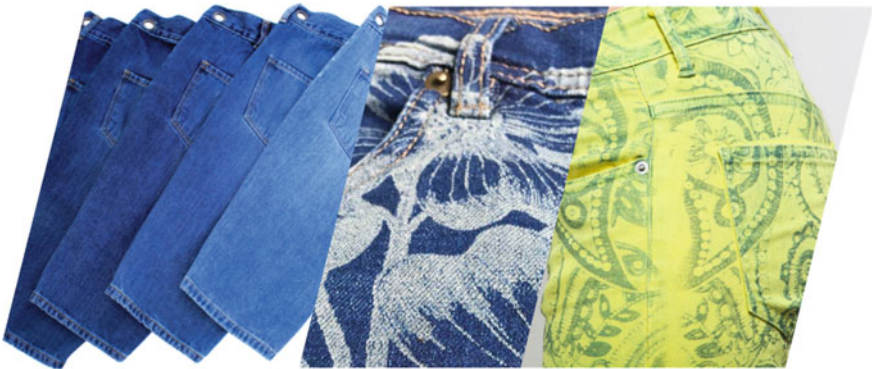
Fig. 4.2 Changes of color by laser local destruction
