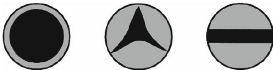
Fig. 2.8 Examples of conductive bicomponent fibers (black indicates conductive component)
