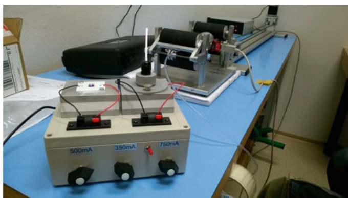
Fig. 5.29 Device for testing of LED effectivity
