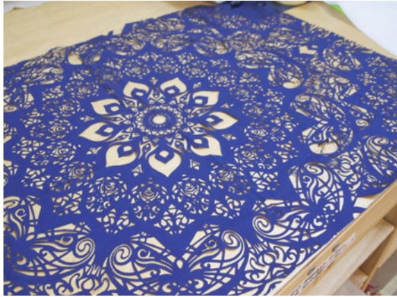
Fig. 8.11 Local cutting of fabric created by CO 2 laser (designed by Zuzana Hrubošová)
