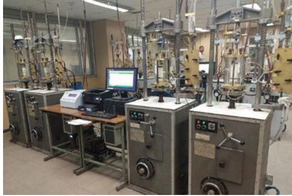
Fig. 6 Semi-automatic triaxial machine in CSMRS, New Delhi
