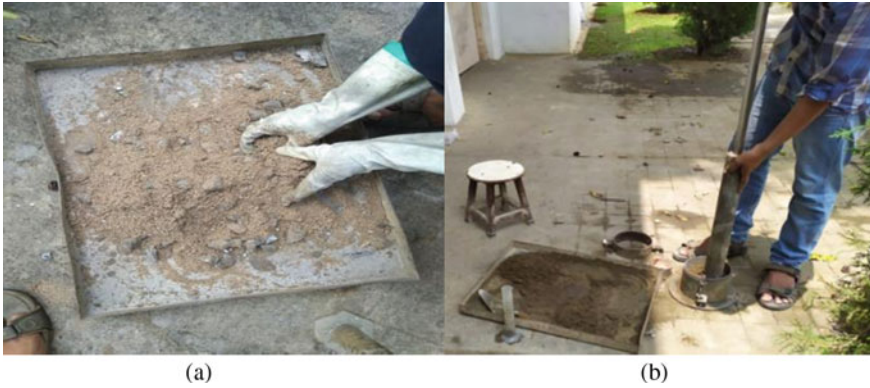
Fig. 1 Sample preparation a mixing b compaction
