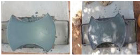
Fig. 3 Plastic waste paver block
