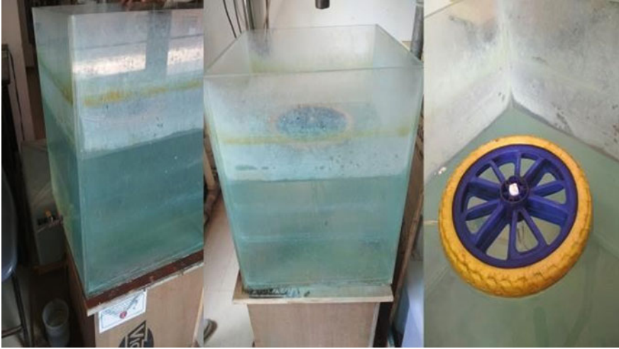
Fig. 4 The various levels of water in water tank and float positions with constant discharge
