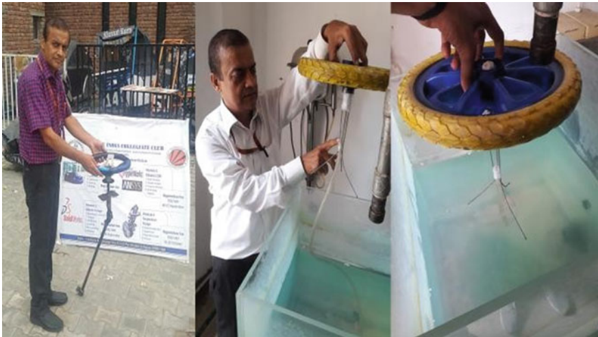
Fig. 2 Theme idea, ingress tube and floating device maintaining constant head
