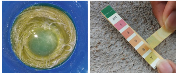
Fig. 1 Soaking of Peepal fibers in NaOH solution and Verifying the PH value
