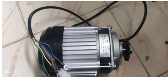
Fig. 3 Brushless DC motor
