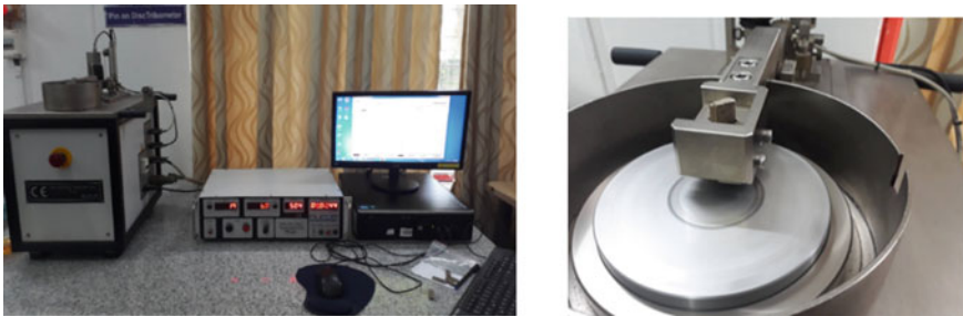
Fig. 1 a Pin-on-disc tribometer set-up. b Specimen set-up
