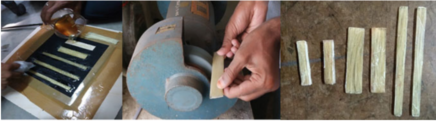
Fig. 2 Pouring of polyester solution into the mold cavity, grinding of samples and final test samples of the composites
