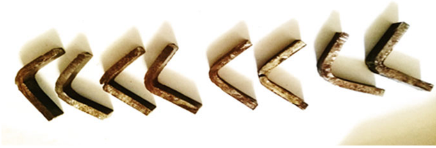
Fig. 5 Specimens after impact failure
