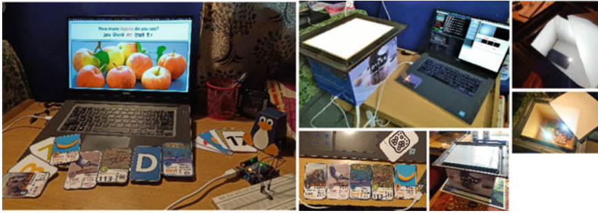
Fig. 4 Showing the game interface with the answer cards (far left), the setup with the box, photo frame, etc., (middle top and middle bottom right) printed cards with fiducial marker at back (middle bottom left), used phones as camera (far right)
