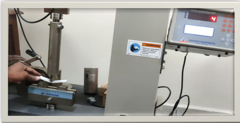
Fig. 9 Specimen removal after failure occurs in flexural testing
