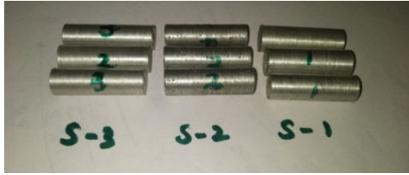
Fig. 4 Wear test specimens, diameter: 10 mm, length: 30 mm
