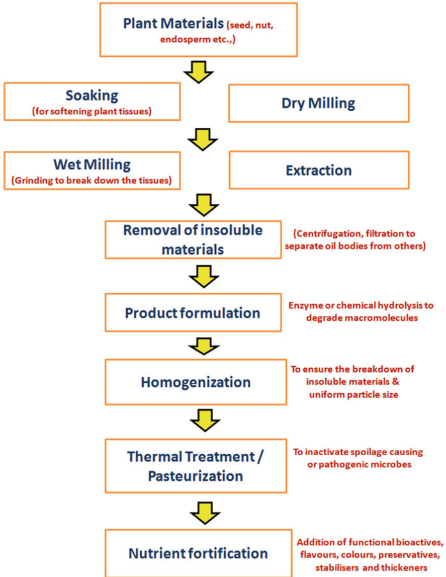
Fig. 5.1 Processing steps involved in the development of plant-based milk alternatives. (Adapted from McClements et al. 2019; Reyes-Jurado et al. 2021)
