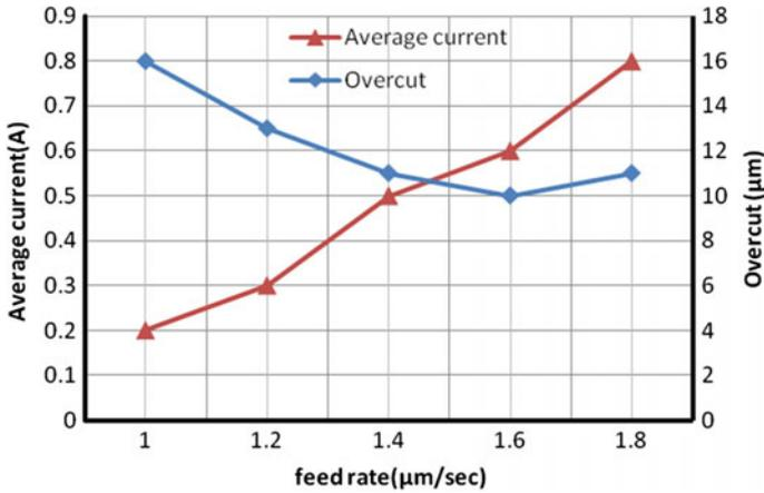
Fig. 3 Influence of tool feed rate on average current and overcut
