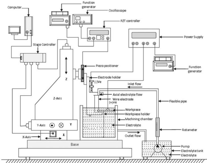
**Fig. 1** Schematic diagram of the WECMM experimental setup
