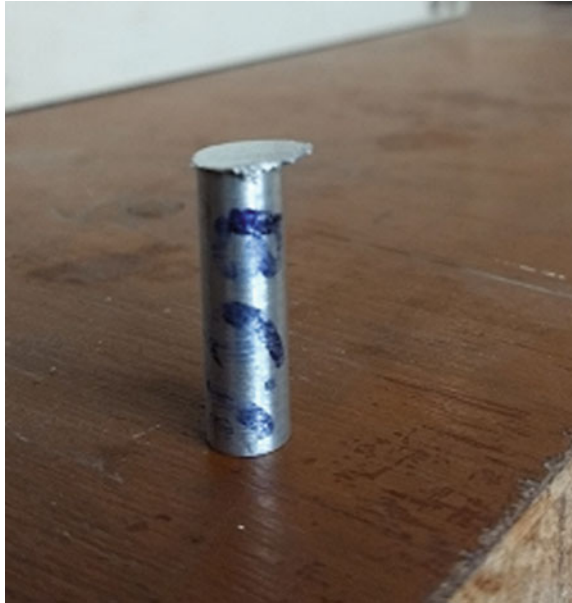
Fig. 8 Thick layer of Al stuck on the contact surface of the pin
