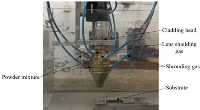
Fig. 1 Setup for direct laser metal layer deposition
