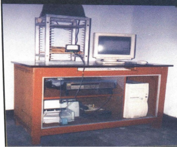
Fig. 1 Arrangement for experiment with MIS device (under illumination for studying volt-ampere characteristics, using Keithley, 238 high source measure units)
