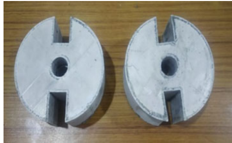
Fig. 5 Fixture/tooling for circular in-line extrusion “die insert” pattern
