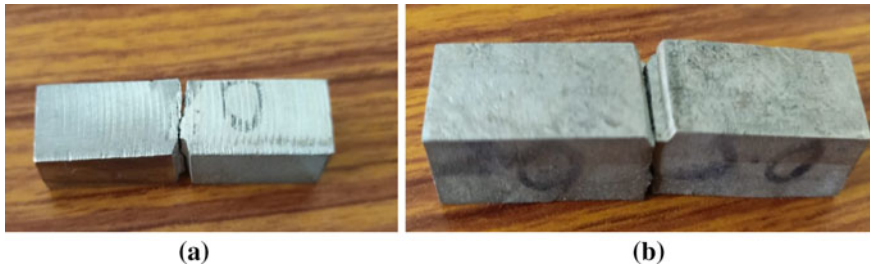
Fig. 8 a As-casted impact tested sample. b AHNC impact tested sample
