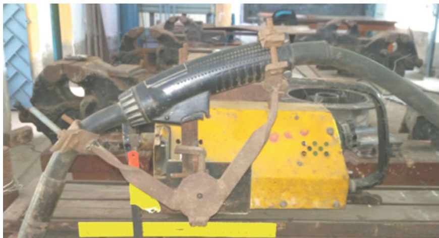
Fig. 2 Welding gun mounted on motor-driven vehicle
