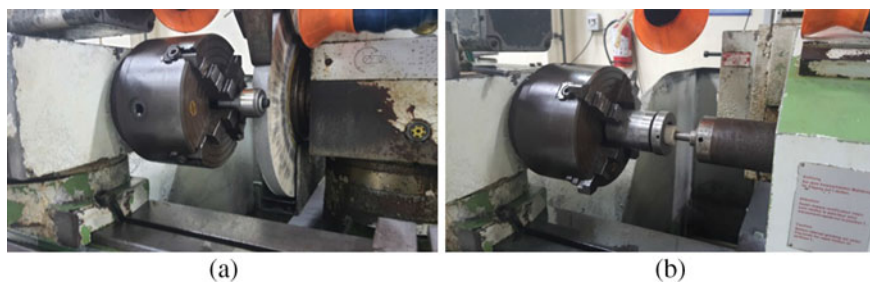
Fig. 2 a OD grinding set up. b ID grinding set up
