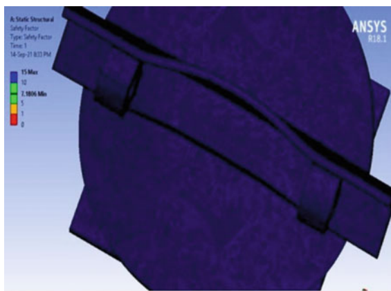
Fig. 9 Mild steel—factor of safety
