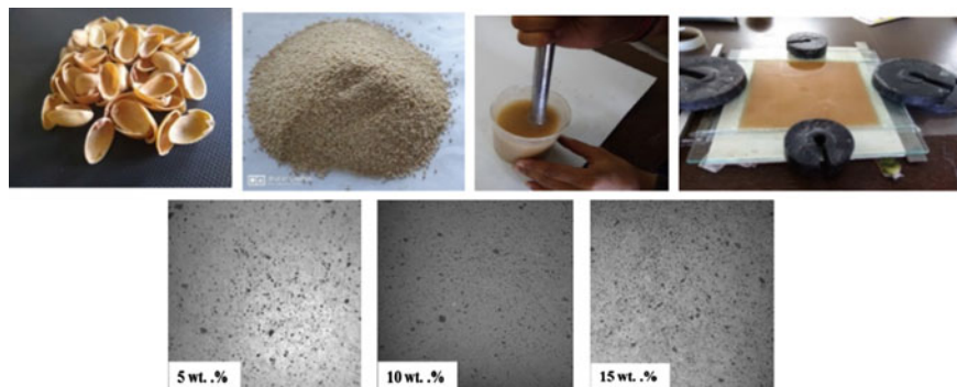
Fig. 1 Preparation of PSF/epoxy composites
