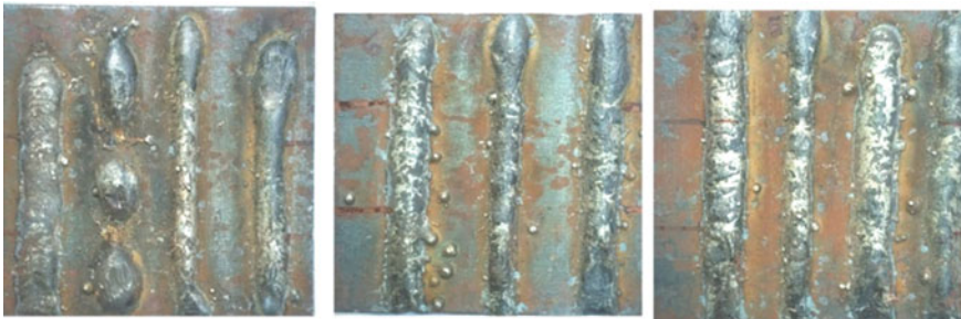
Fig. 3 Bead on plate during trial runs
