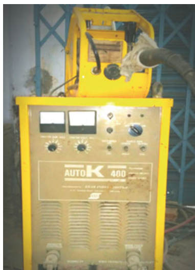
Fig. 1 ESAB, India made auto K 400 GMAW machine
