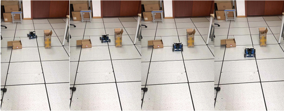
Fig. 3. An example of Opt_TEB obstacle avoidance trajectory
