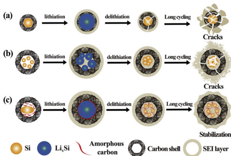
Fig. 13 Schematic illustration of lithiation and delithiation processes of (a) Si@C, (b) traditional yolk-shell Si@void@C and (c) as-prepared industrial Si@void@C with interconnected porous carbon network. Reprinted with permission from Jiao et al. (2018), copyright (2021) © Elsevier
