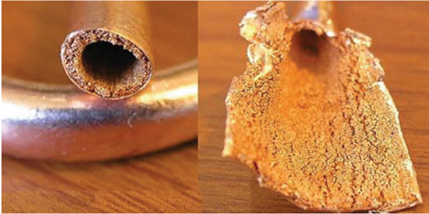
Fig. 4.9 Wick with sintered structure (Elnaggar 2016)
