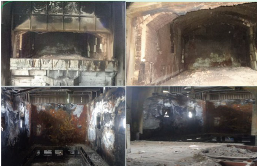
Fig. 2.7 Furnace before kaizen
