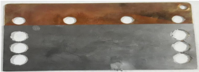
Fig. 11.9 A photograph of the current collector with carbon coating
