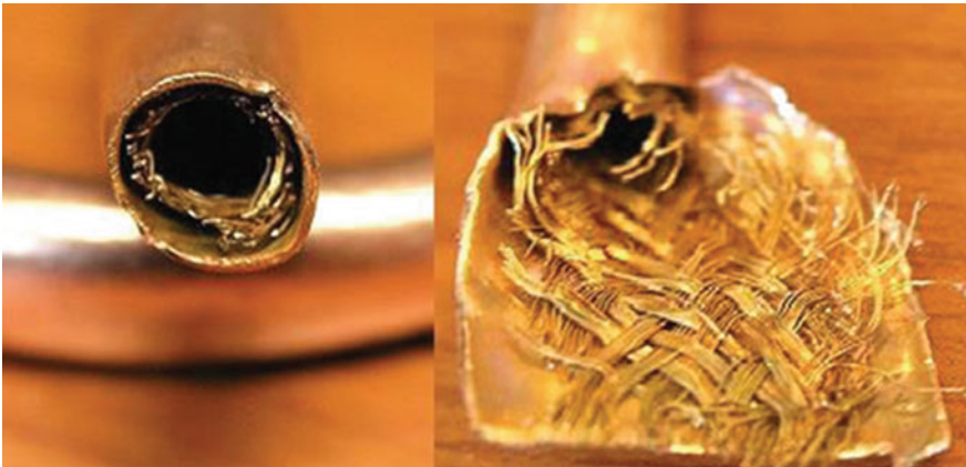
Fig. 4.11 Screen mesh wick (Elnaggar 2016)
