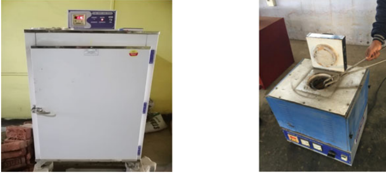
(a) Hot air oven (for moisture determination) (b) Furnace (for VS and AC determination)
