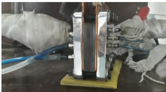
Fig. 11.16 Single cell fuel cell on test station
