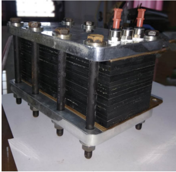
Fig. 11.10 A photograph of the PEMFC stack used in the present study
