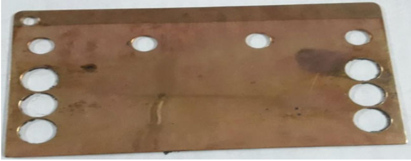
Fig. 11.8 A photograph of the current collector without carbon coating
