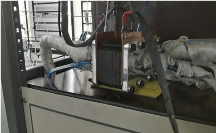
Fig. 11.20 Ten stack PEMFC on test station
