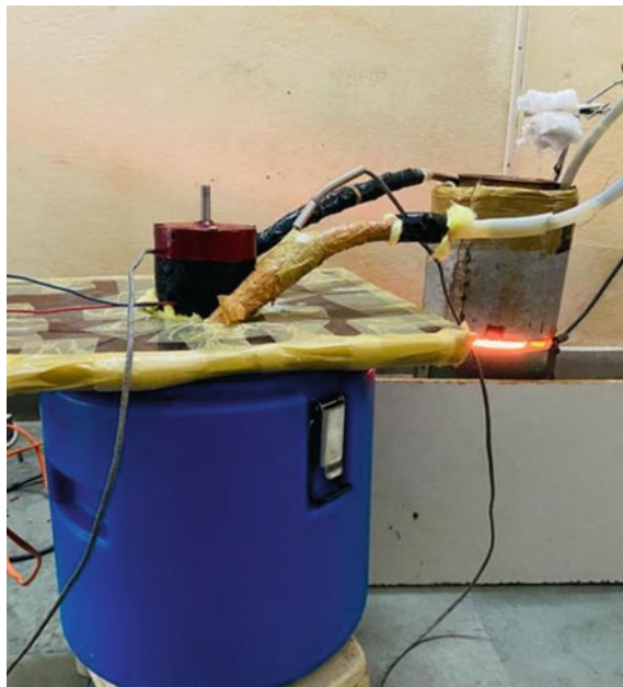
Fig. 2 Lab scale testing set-up with commercial heat storage system
