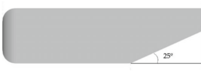
Fig. 1 Ahmed body with diffuser angle of 25^\circ
