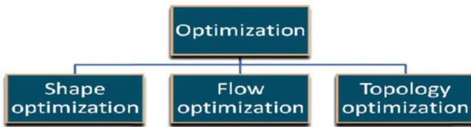
Fig. 8 Optimization approach in micro-mixers
