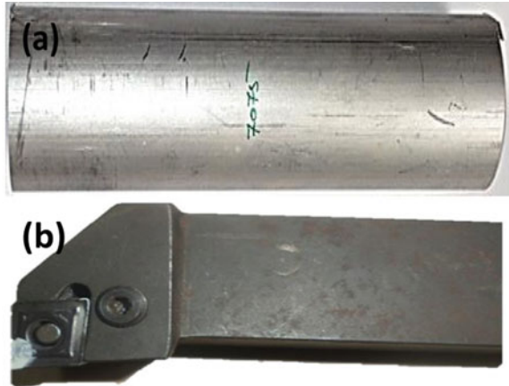
Fig. 1 Images of a Al 7075 workpiece for turning and b Cutting tool with tool holder
