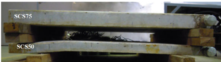
Fig. 8.11 Comparison of permanent deformation of SCS50 and SCS75 sandwich panels after test, reprinted from Wang et al. (2015a), copyright 2022, with permission from Elsevier
