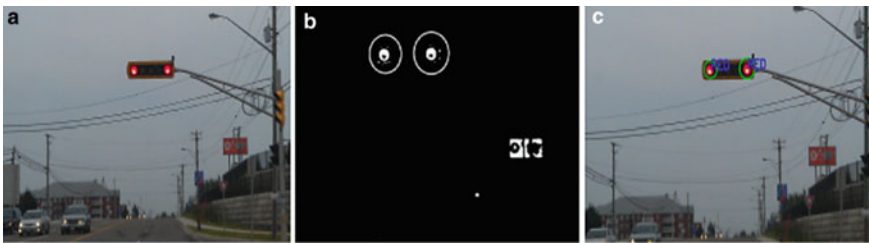
Fig. 2 a Raw image. b Color mask. c Result detection
