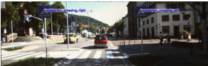
Fig. 3 Street sign detection using the color-based approach
