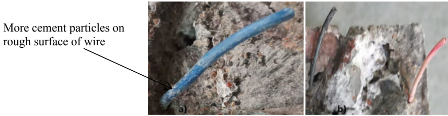
Fig. 8 Comparison between rough and non-rough surface of wire
