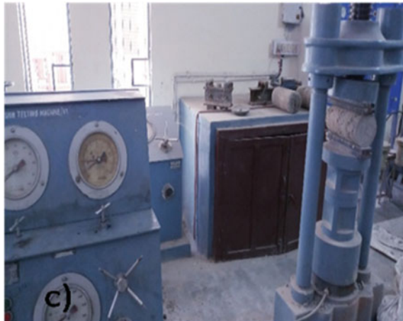
Fig. 5 Splitting tensile test set-up
