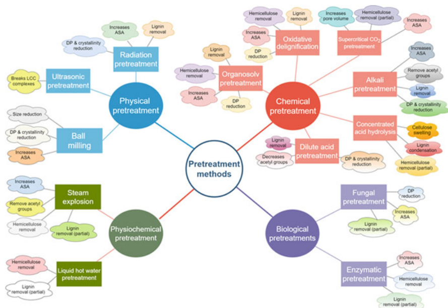
Fig. 2.8 Schematic representation of changes induced after pretreatment of lignocellulosic biomass
