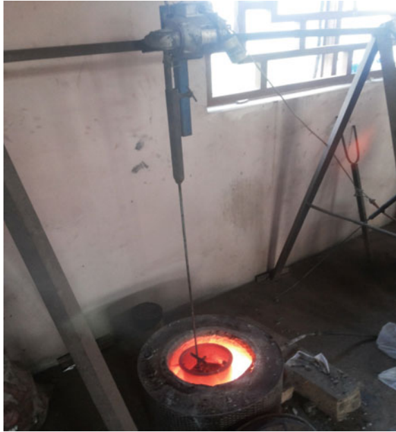
Fig. 2 Mechanical stirring setup for the Al6063-based composite slurry
