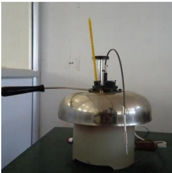
Fig. 3 Pensky–Marten flash apparatus
