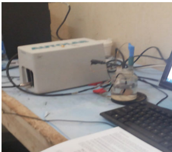
Fig. 6 Electrochemical tests setup using AUTOLAB PGSTAT 204 N
