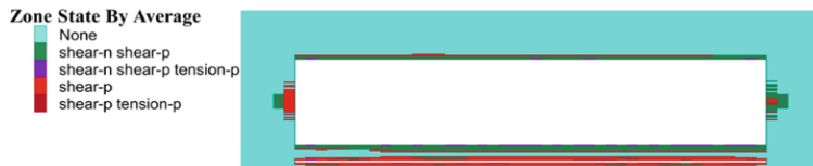
(c) coal pillar width 30m
