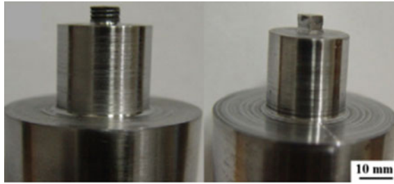
Fig. 4 Tools with two different pin shapes/geometries [11]
