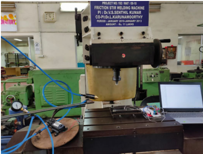
Fig. 2 In-process spray cooling assisted friction stir welding setup
