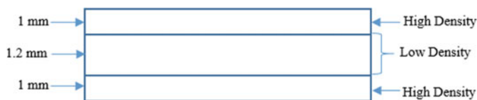
Fig. 5 Density configuration of the BiS along its cross-section
