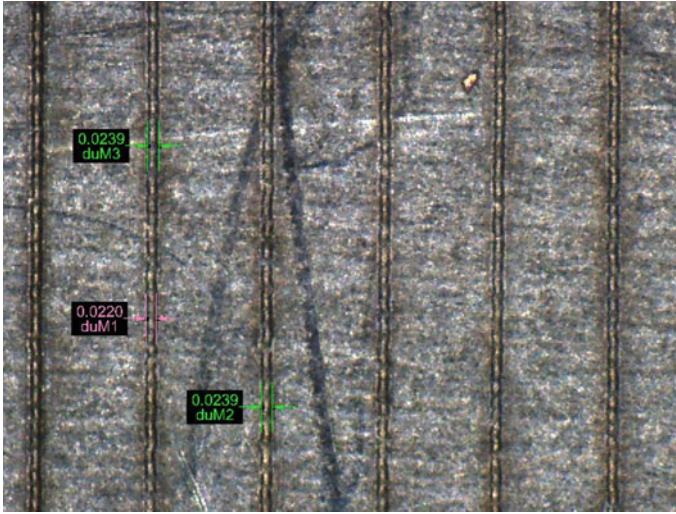
Fig. 7 Minimum kerf width (in \mu\text{m} ) received for nanosecond laser NUQA-1064-NA-0030-YZ
