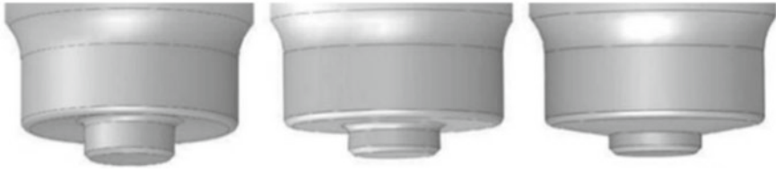
Fig. 15 Concave, flat and convex shoulder profiles [41]
