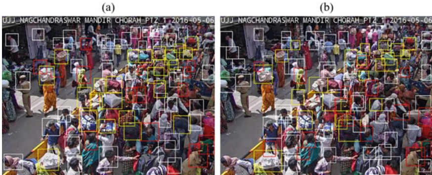
Fig. 5 Bounding boxes (a) in the ground truth and (b) by model prediction. White, Red, and yellow boxes represent male, female, and head luggage class, respectively
