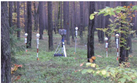
Fig. 3 TLS measurements and output in a forest circular sample
