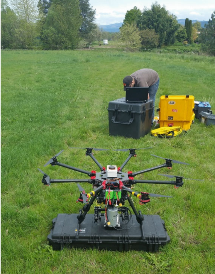
Fig. 2 Velodyne HDL-32 LiDAR sensor (silver cylinder on bottom of aircraft) mounted on a DJI s1000 quadcopter
