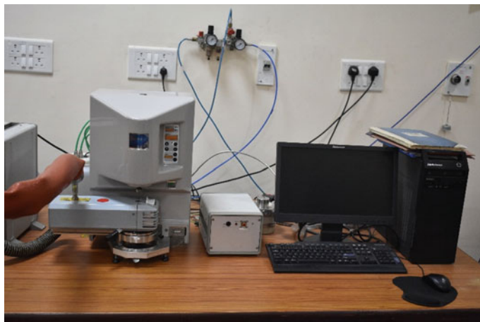
Fig. 3 Advanced air bearing rheometer Bohlin Gemini 2
