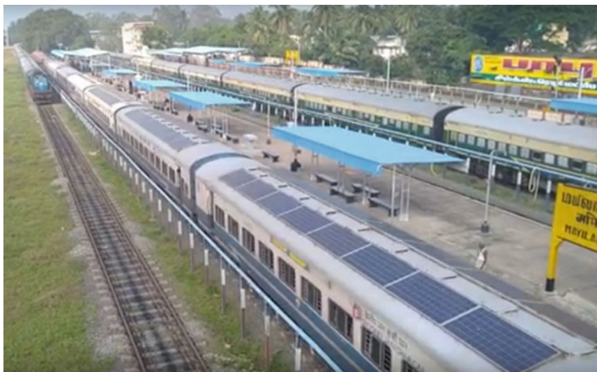
Fig. 13 PV cell mounted on the roof of Coimbatore-Mayiladuthurai Jan Shatabdi Express train
