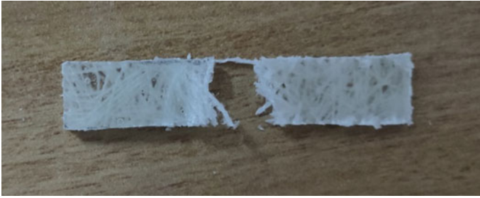
Fig. 7 Impact test fractured specimen
