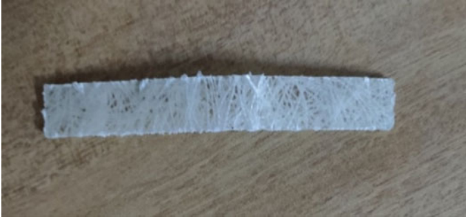
Fig. 6 Flexural test fractured specimen
