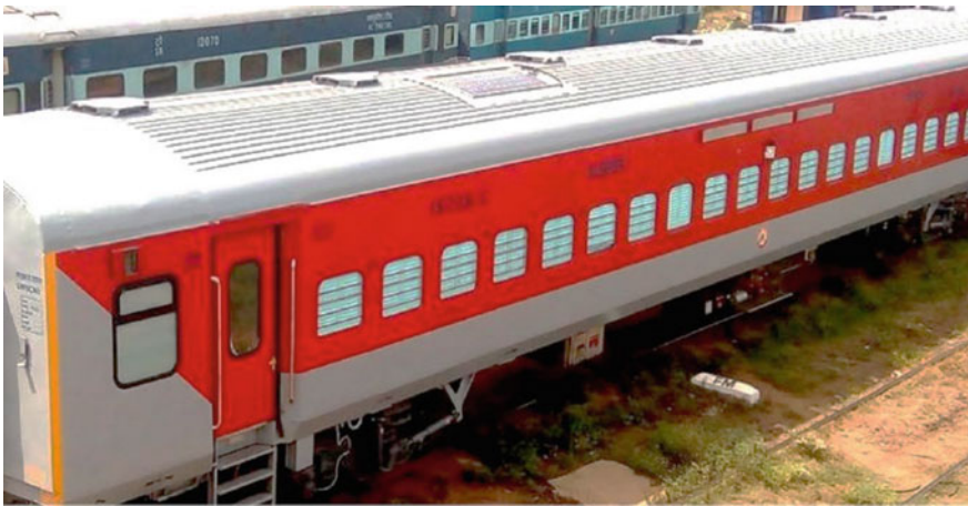
Fig. 10 A sleeper class LHB coach fitted with two flexible solar panels
