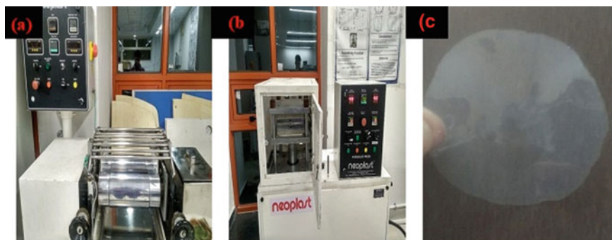
Fig. 1 Pictorial view of a hydraulic press, b two-roll milling machines, and c prepared transparent ZnO film
