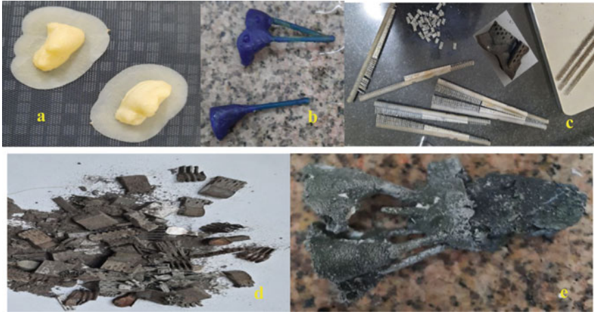
Fig. 3 a Pattern for IC prepared by recycled ABS, b wax pattern, c DMLS-based parts fabricated showing support structure, d collected wastes from 3D metal printing process, and e final IC parts of DC from 3D printing metal wastes
