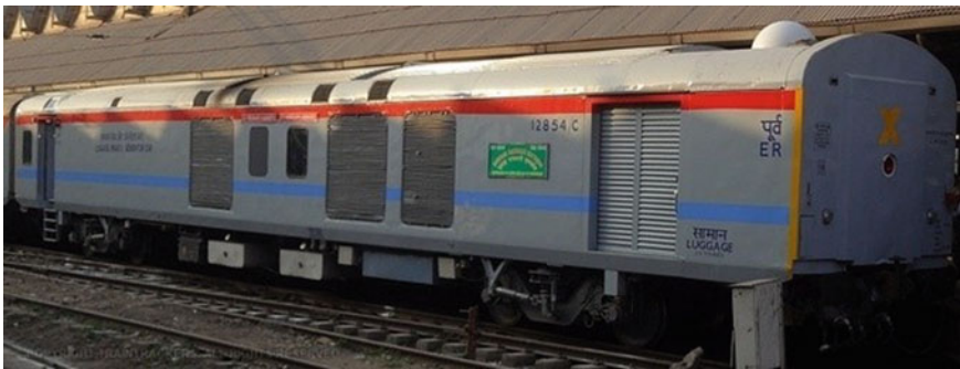
Fig. 2 LHB luggage brake and generator car
