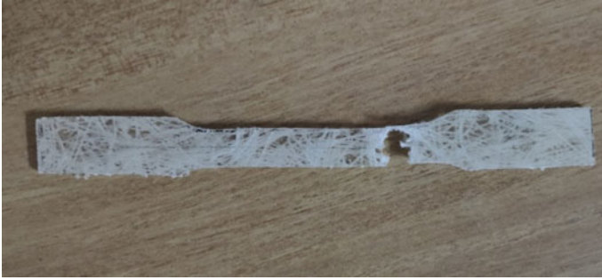
Fig. 5 Tensile test fractured specimen
