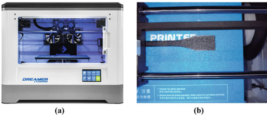
Fig. 2 a and b Dreamer FDM 3D printer. Tensile test specimen printing process
