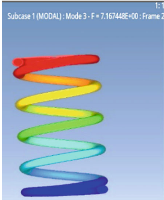
Fig. 14 Modal analysis for helical spring showing frequency is calculated to be 7.16 Hz
