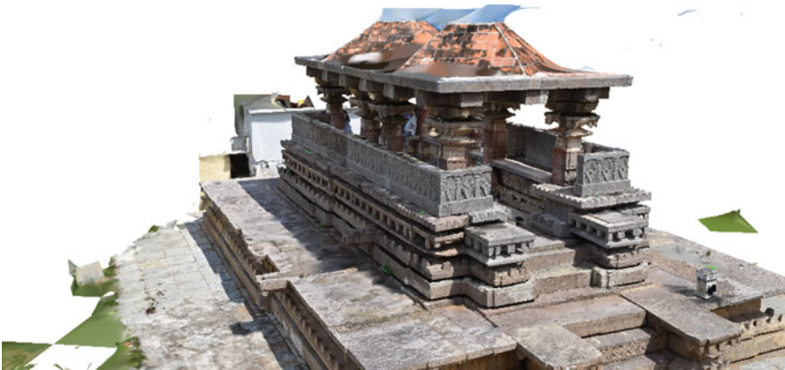
Fig. 2 Raw data (Textured) obtained after uploading to reality capture
