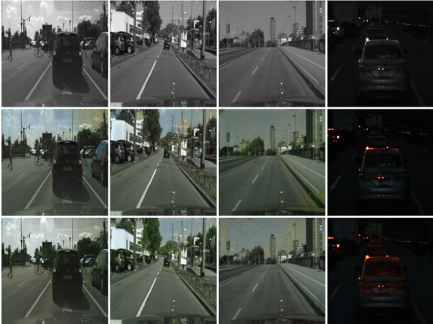
Fig. 1 Outputs of image to image translation from monochrome to RGB. 1st row: the input images, 2nd row: the generated images using CycleGAN model [35], and 3rd row: the generated images using CUT model [26]
