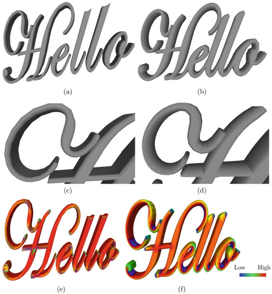
Fig. 9 (Best viewed in colour) Qualitative comparison 3D mesh from a Blender [5], b Our method, c Zoomed-in region of mesh in (a) , d Zoomed-in region of mesh in (b) , e Blender output's Gauss curvature and f Our output's Gauss curvature
