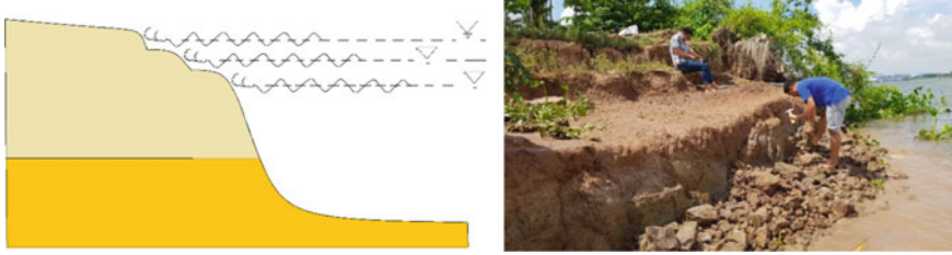
Fig. 14.17 Erosion mechanism of riverbanks in an Giang province, Vietnam
