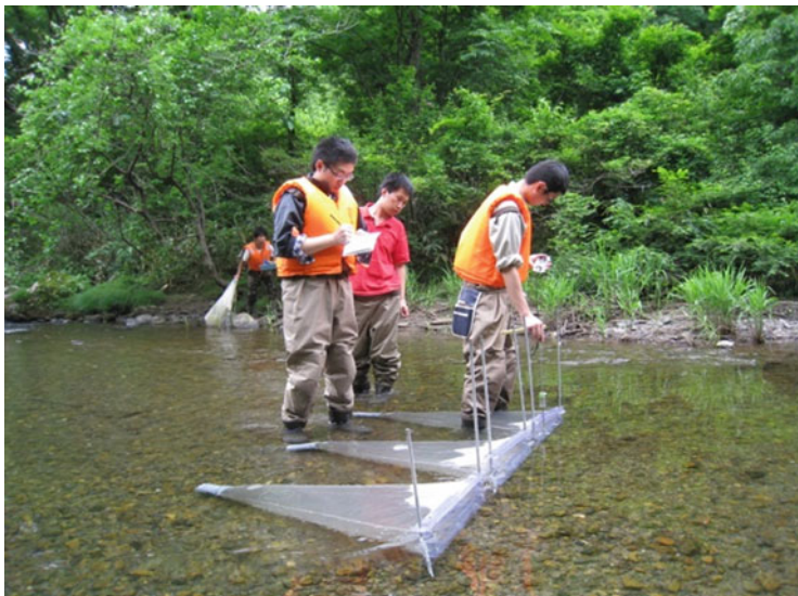
Photo 7.3 Particulate organic matter sampling for evaluation of water quality responses to dam construction and operation (photo taken by the author)
