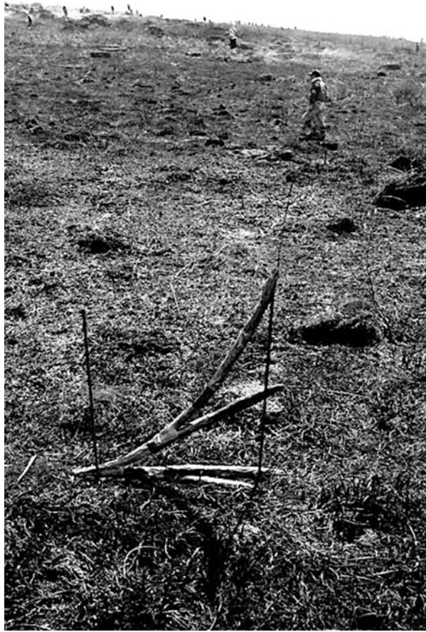
Photo 5.2 A system for measuring the burning temperature of grasslands
