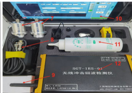
(b) Wireless impact echo detector
