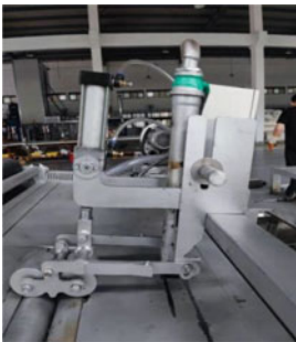
(a) Internal welding
