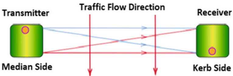
Fig. 3 Vehicle detection mechanism
