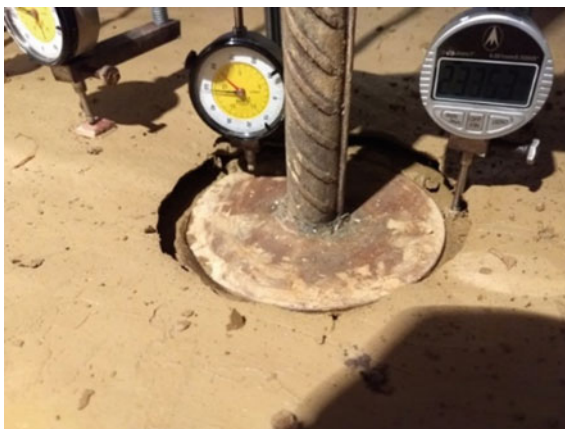
Fig. 3 Settlement of footing in the soil bed
