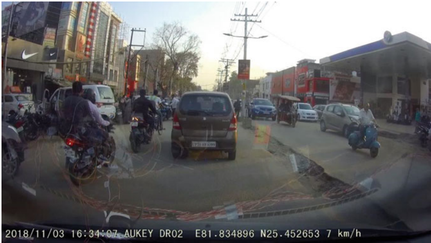
Fig. 5 Video grab of traffic scenario captured using GPS equipped dash camera installed in probe vehicle
