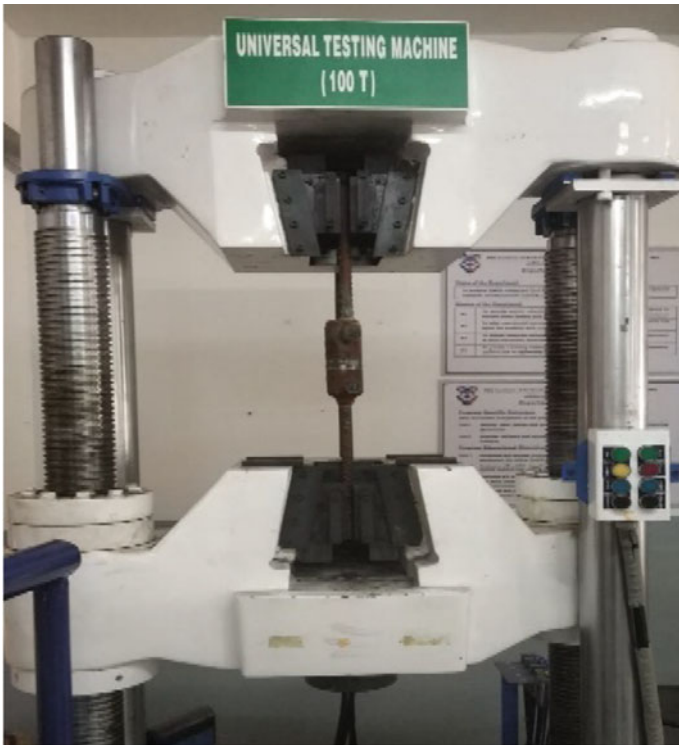
Fig. 3 The specimen under tension loading
