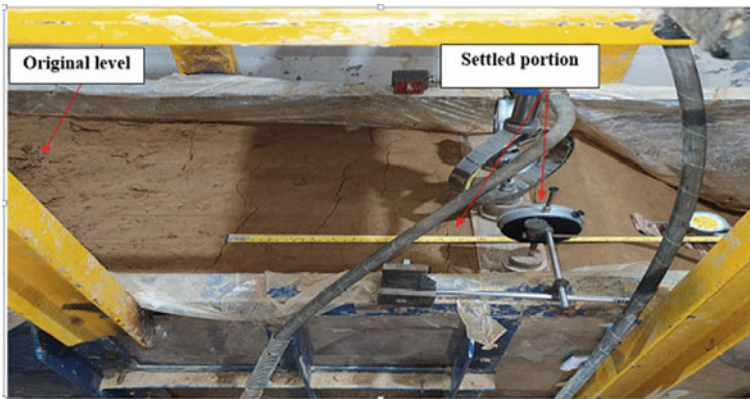
Fig. 2 Picture of experimental setup for foundation placed at 1B
