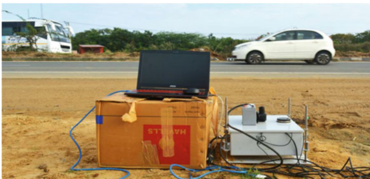
Fig. 4 Setup of the TIRTL instrument
