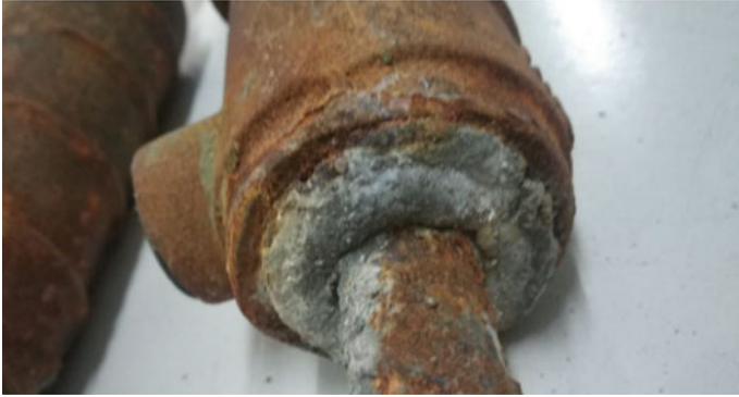
Fig. 4 Bond failure in the specimens
