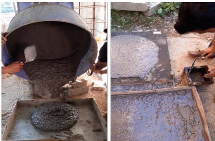
Fig. 1 Preparation and placement of SCGPC
