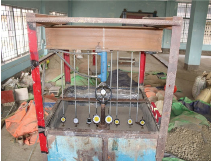
Fig. 2 Test setup (model plate load test)
