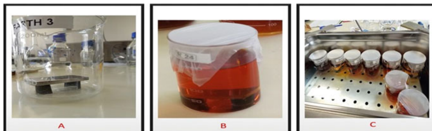
Fig. 2 Experimental setup, sample setup (a), immersed sample in glass beaker (b), samples are in water bath (c)
