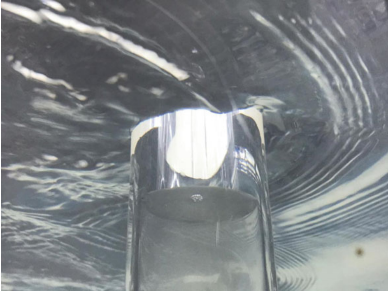
Fig. 8 Vortex formed at 4 rotations. The water strikes the pier directly and spreads up in three different directions (three-dimensional flow, time interval 10 min)
