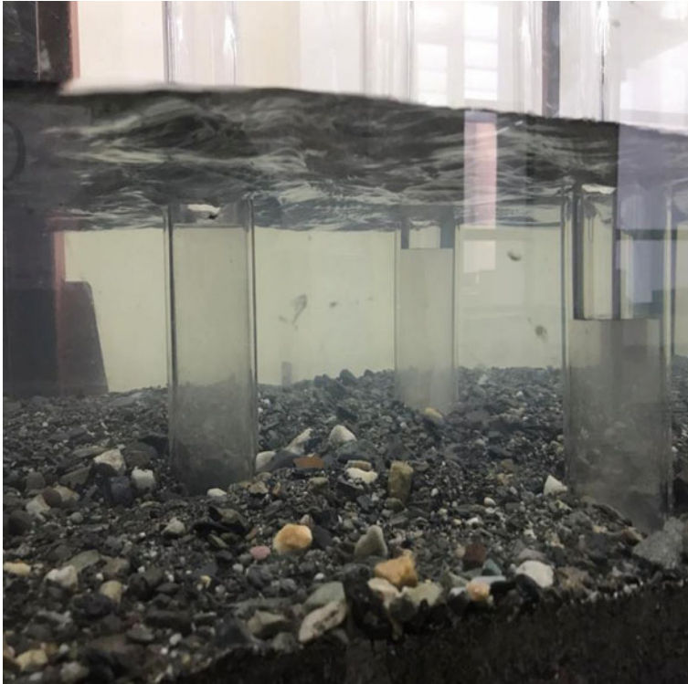
Fig. 7 Arrangement of piers in triangular pattern with c/c distance 20 cm (time interval 10 min)
