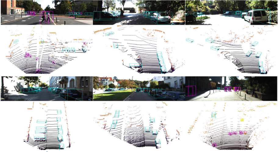
Fig. 4. Qualitative results on the KITTI test dataset using LGDA-GNN. We show the predicted 3D bounding box of Cars (green), Pedestrians (red) and Cyclists (blue) on both the image and the point cloud. Best viewed in color.
