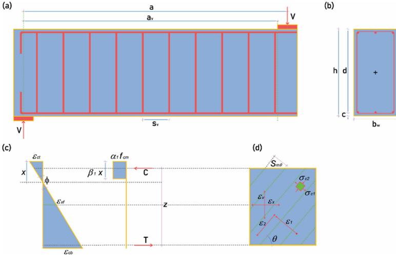
Fig. 1. a) Lateral view and b) cross-section of the RC beam. c) Flexural and d) Shear model.
