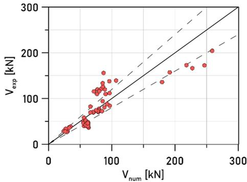
**Fig. 2.** Comparison between the experimental and numerical shear strength.
