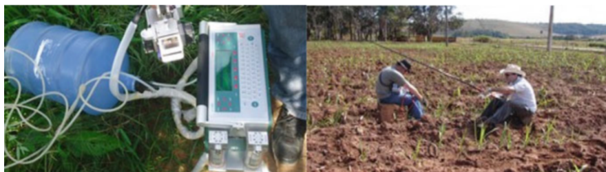
Fig. 16.5 (a) Infrared Gas Analyzer (IRGA) and (b) its application under field conditions to assess the physiological performance of sugarcane genotypes following pre- or post-emergence herbicide application. (Photo source: Evander A. Ferreira)
