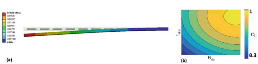
Fig. 3 a Comparison between original and displaced geometry for the optimized design point and b Variation of coefficient of lift with No. of ribs and skin thickness
