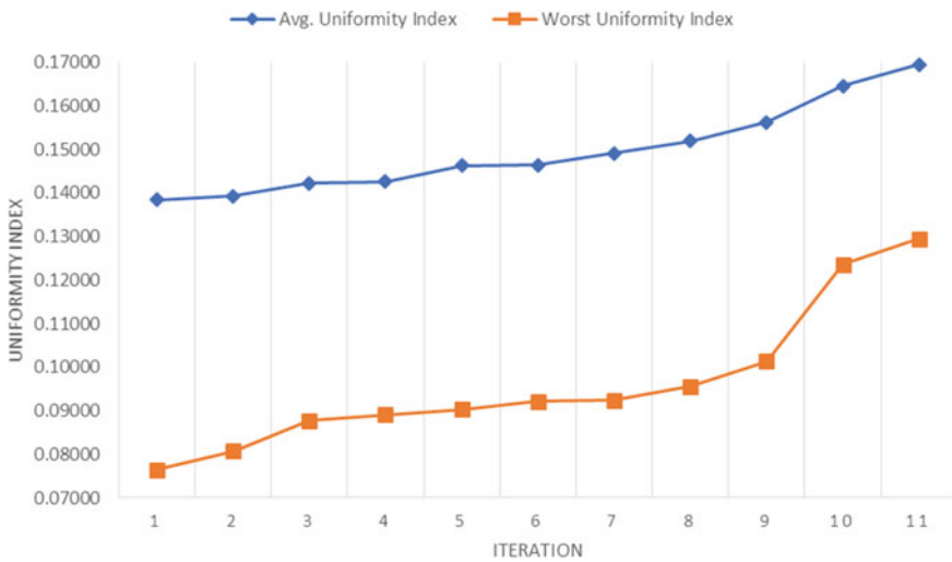
Fig. 8 Performance corresponding to centroid and worst point of the Box complex for different iterations
