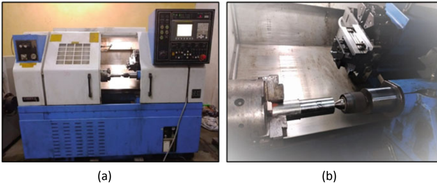
Fig. 1 a CNC turning centre used for experimentation. b Arrangement of tool, workpiece and dynamometer force sensor plate
