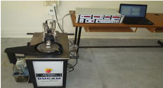
Fig. 4 Pin-on-disk machine for wear test machine
