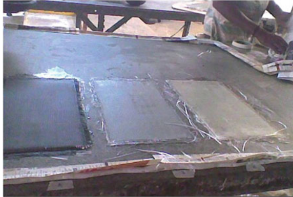
Fig. 3 Digital photo of B-E composite containing different fillers after post-curing
