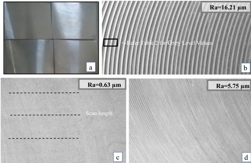
**Fig. 2** Photographs of the specimens and images captured using the proposed setup
