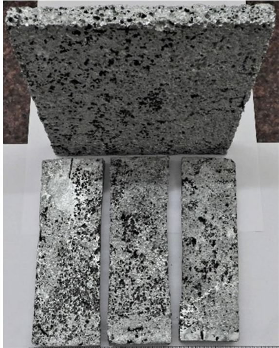
Fig. 4 Examples of metallic foams processed by liquid-state processes
