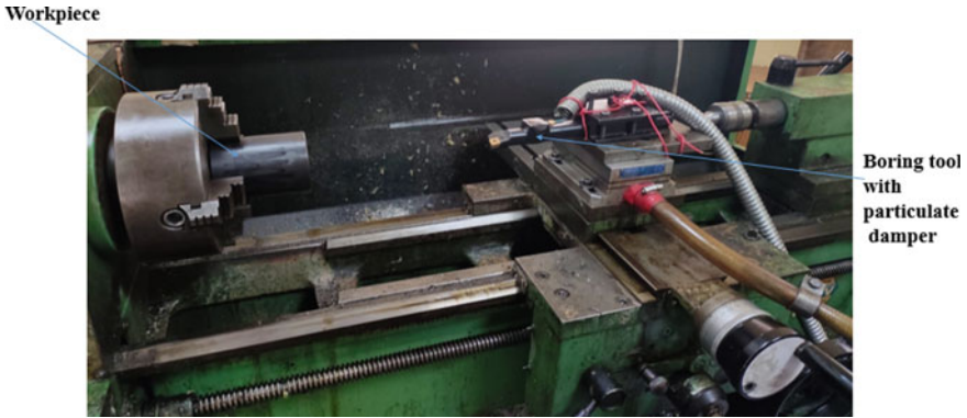
Fig. 2 Photograph of the boring bar with particulate damper
