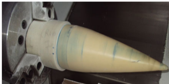
Fig. 4 Holding fixture for external machining of radome
