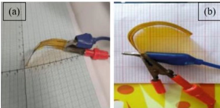
Fig. 5 Actuator of varying dimension: a 7 \times 2 and b 5 \times 2\ \text{cm}^2
