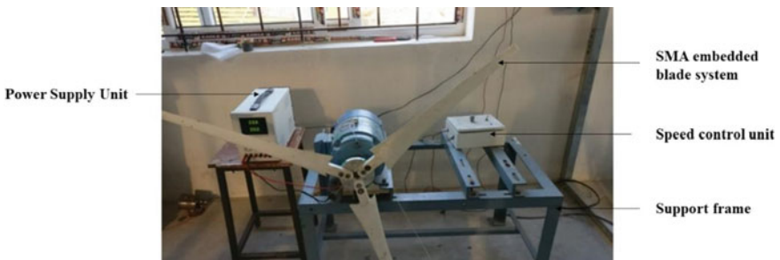
Fig. 12 Experimental setup for active vibration control of the blade
