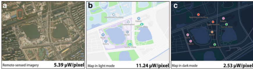
Fig. 22.2 A comparison of the energy consumption of map and remote-sensed imagery; a remote-sensed imagery; b a map in light mode; and c a map in dark mode with the same map data
