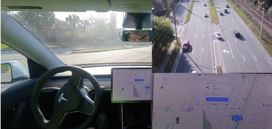
Fig. 35.5 Tesla’s “Full Self-Driving Beta” guided by the HD map during a left turn in real traffic ( https://youtu.be/uClWIVCwHsI from 2021.04.11)
