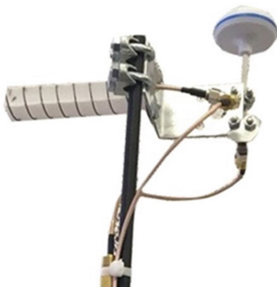
Fig. 8 Circular-polarized antenna system
