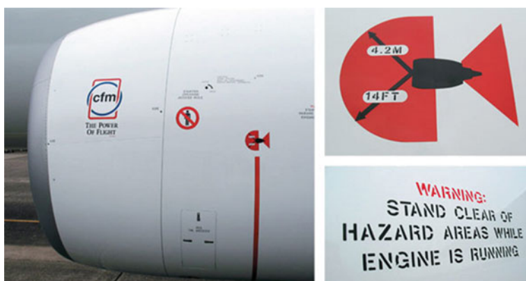
Fig. 3 Hazardous areas of gas turbine engine [tacomaworld.com]
