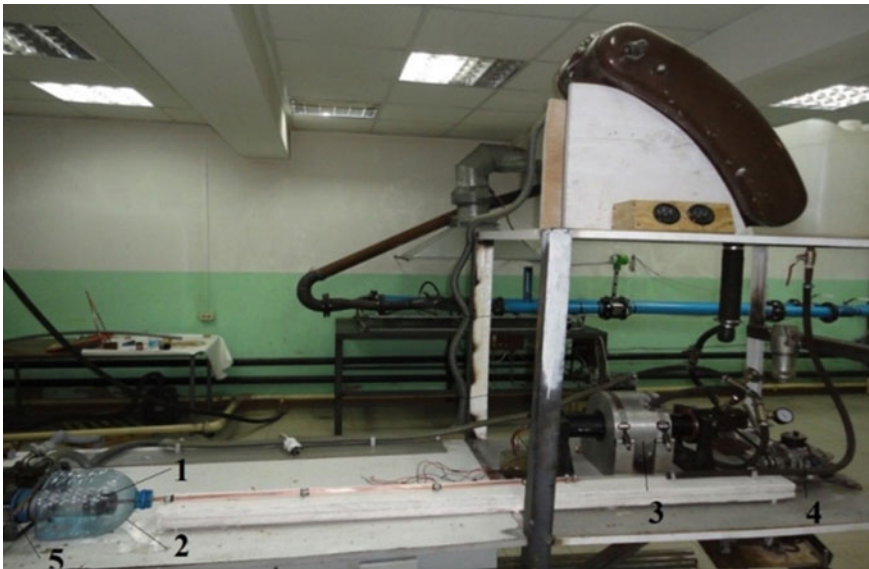
Fig. 4 Experimental setup for investigating the characteristics of the oil pipe: 1—oil distribution sleeve; 2—protective casing; 3—oil pump electric motor; 4—oil pump; 5—electric drive of oil distribution sleeve
