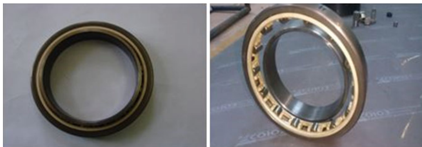
Fig. 7 Inter-shaft roller bearing
