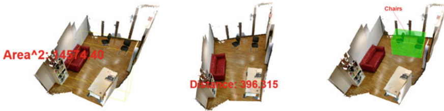
Fig. 2 Example of user-based annotations of an indoor point cloud. These annotation operations are recorded as blockchain data in the presented case study, using the prototypical PDL software component
