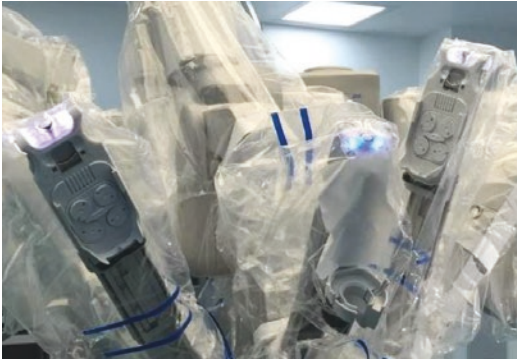
Fig. 7 Control and Clutch with LED indicator ON to proceed
