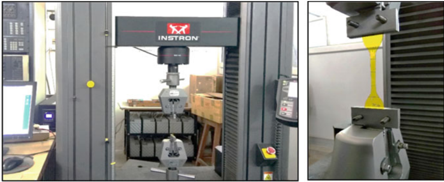
Fig. 4 Experimental setup (INSTRON UTS 5982)
