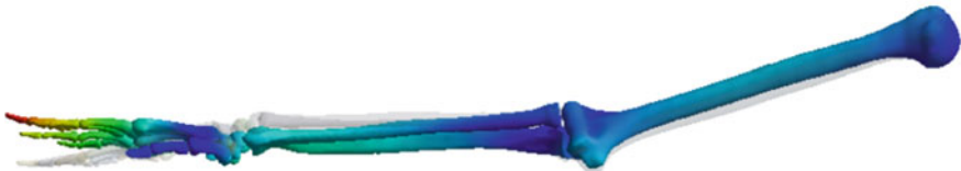
(c) Third Natural Frequency = 165.58 Hz
