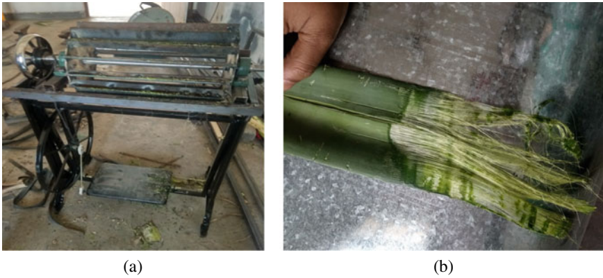
Fig. 6 a Prototype of sisal fibre extracting machine, b sisal fibre obtained from the developed machine
