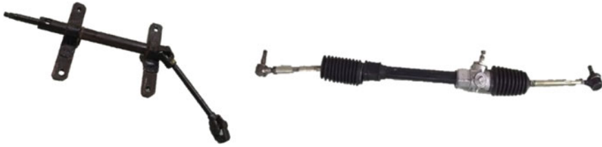
Fig. 2 Steering column and rack used for the rig testing
