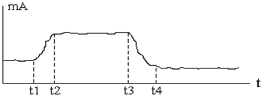
Fig. 4. The output waveform of the vibration transmitter when the acceleration sensor is installed on the rear axle
