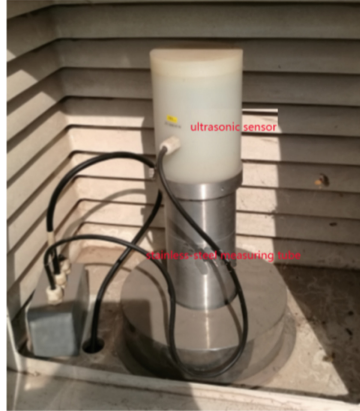
Fig. 2. The measurement part of the evaporation sensor
