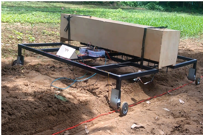
Fig. 10. The real model of a mobile robot for spinach water seed planting
