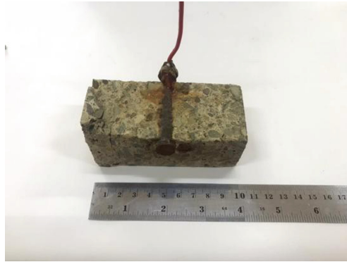
Fig. 6. Corroded reinforcing steel for corrosion potential analysis
